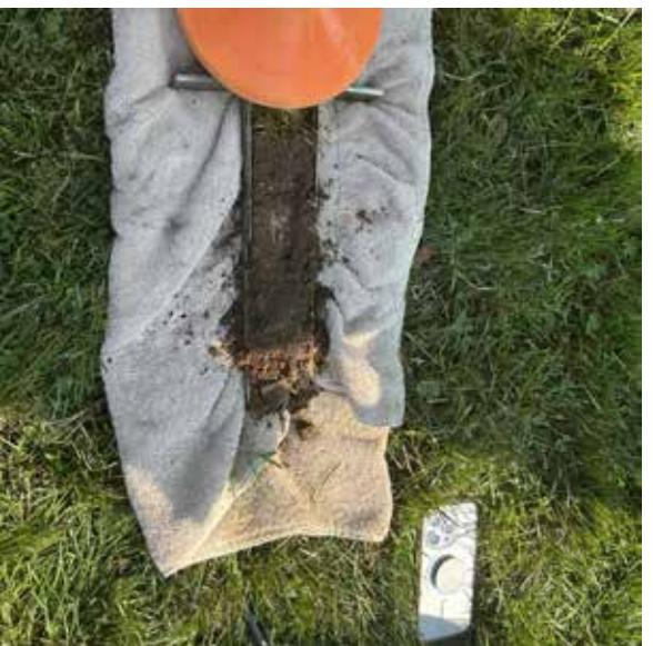
Test point 5 profile showing good root depth and root zone medium depth.
