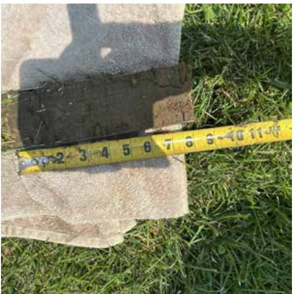
*Test point 2 soil profile showing depth of rootzone medium and root depth*
