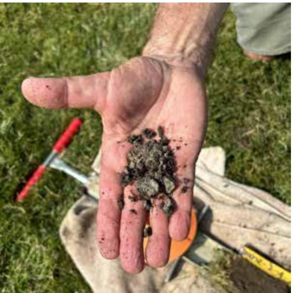
Clay material near base of profile at test point 4
