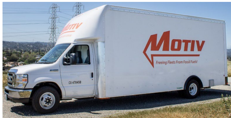
An all-electric box truck adds an electric powertrain to a Ford E-450 chassis. Manufacturer photo.
